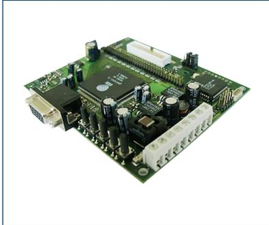
The AKV 03 interface adapts analogue VGA-, SVGA-, XGA and SXGA information to digital LC- Displays. Standard timings such as VGA, SVGA, XGA and SXGA are scaled to the maximum pixel resolution of a connected display module. Downscaling is possible with loss of picture quality.
